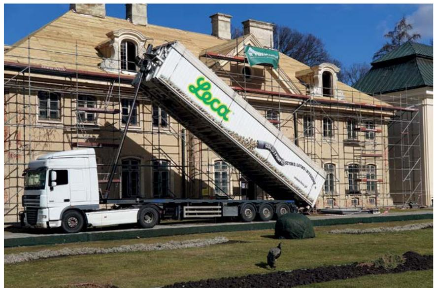
**Vehicle with a pump** for feeding aggregate.
